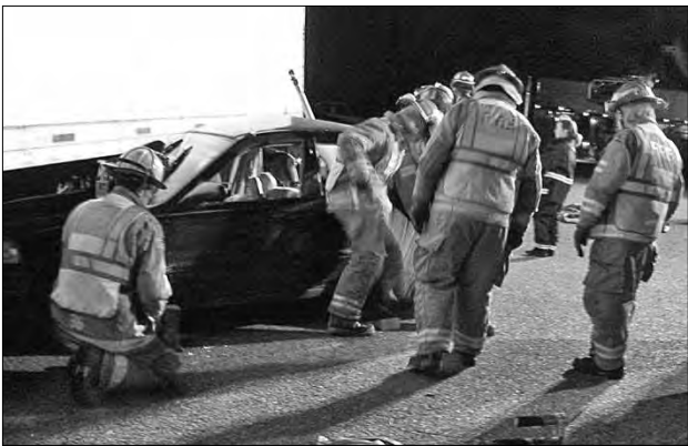
Firefighters work to stabilize a vehicle pinned under the side of a tractor trailer unit.
