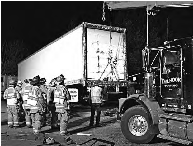
Tailhook's heavy duty wrecker lifts the back of a trailer off a vehicle pinned underneath.
