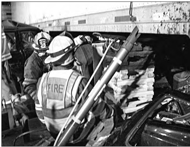
Cribbing (blocks) are stacked up, in a criss-cross pattern, to the bottom of the trailer. An airbag is placed on top of the blocks, just under the trailer floor, to lift the trailer off the vehicle.
