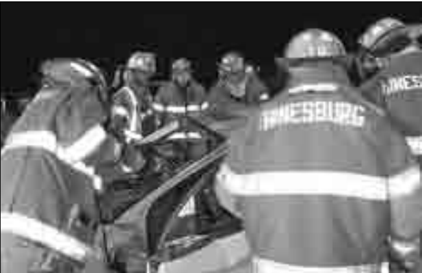
The posts are cut in preparation for removal of the vehicle roof.
