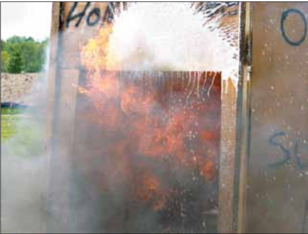
Five minutes into burn, the room has flashed over and is fully involved with flames rolling out the front. Firefighters sprayed foam on the fire to keep it under control
