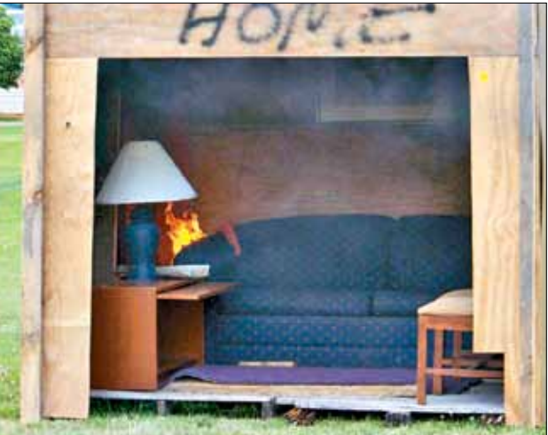
Within two minutes of being lit, smoke is filling the ceiling area and the furniture near the waste basket is burning.
