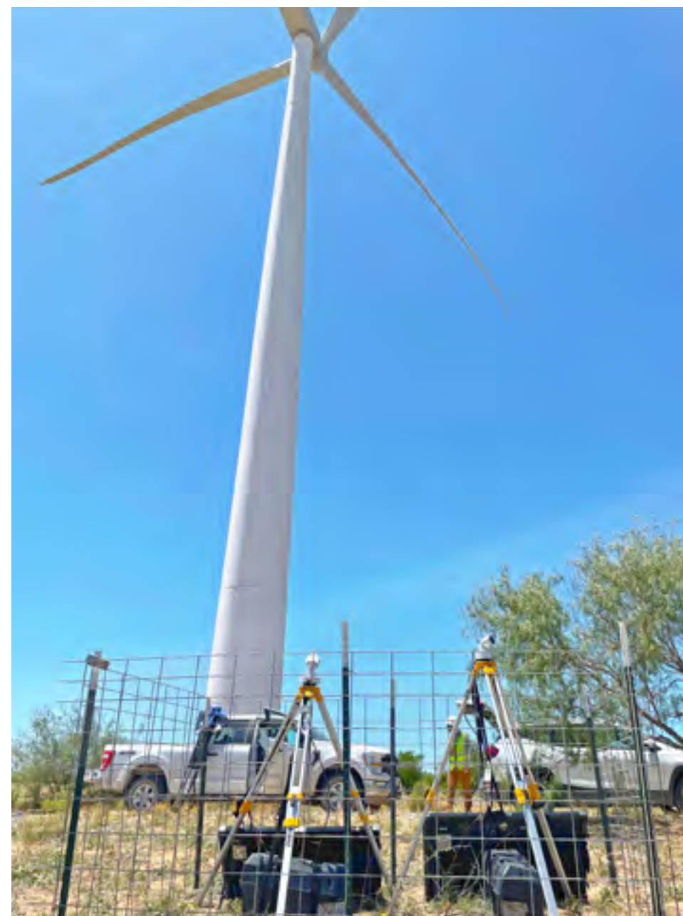
A typical installation of monitoring equipment near a wind turbine.
